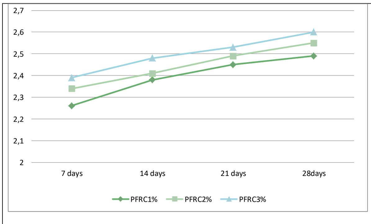
**Figure: (b)** compression of compressive strength m-30 PFRC & conventional concrete of PFRC1%, PFRC2% & PFRC3%.
