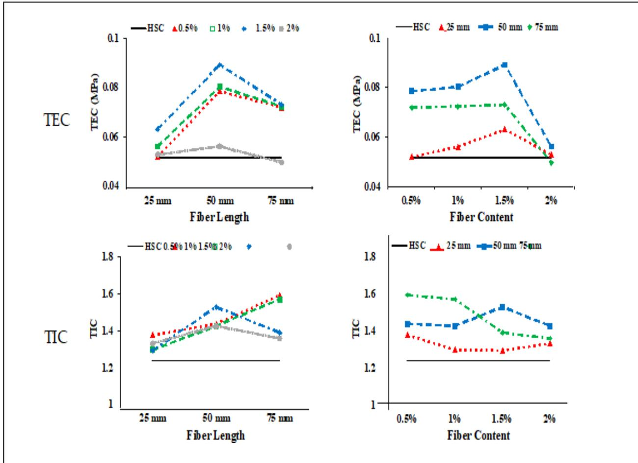
**Figure :-** Influence of coconut fiber on PEC, CEC, TEC, and TIC: (a) Length; (b) Content.
