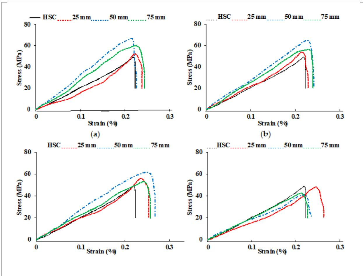
**Figure:** (a) Stress-strain curves for HSC and CFR-HSC with (a) 0.5%, (b) 1%, (c) 1.5%, and (d) 2% fiber content.
