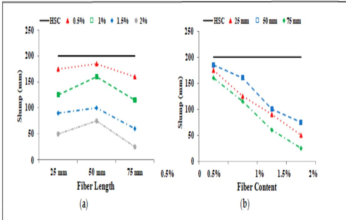
Figure 4.2. Influence on slump: (a) Fiber length; (b) Fiber content.
